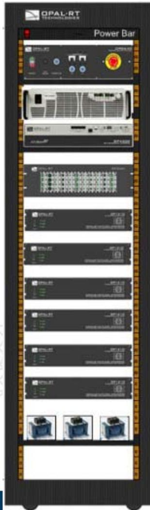
**OP1200** – Fully integrated MMC Test Bench
