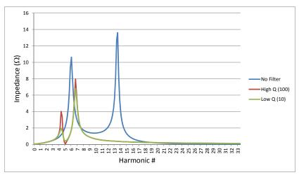
Filter eliminates  $5^{th}$  resonance, but creates new ones that could be as bad (or worse). Best solution probably to split 600 kvar into 2x300 kvar and make two filters— $5^{th}$  and  $7^{th}$
