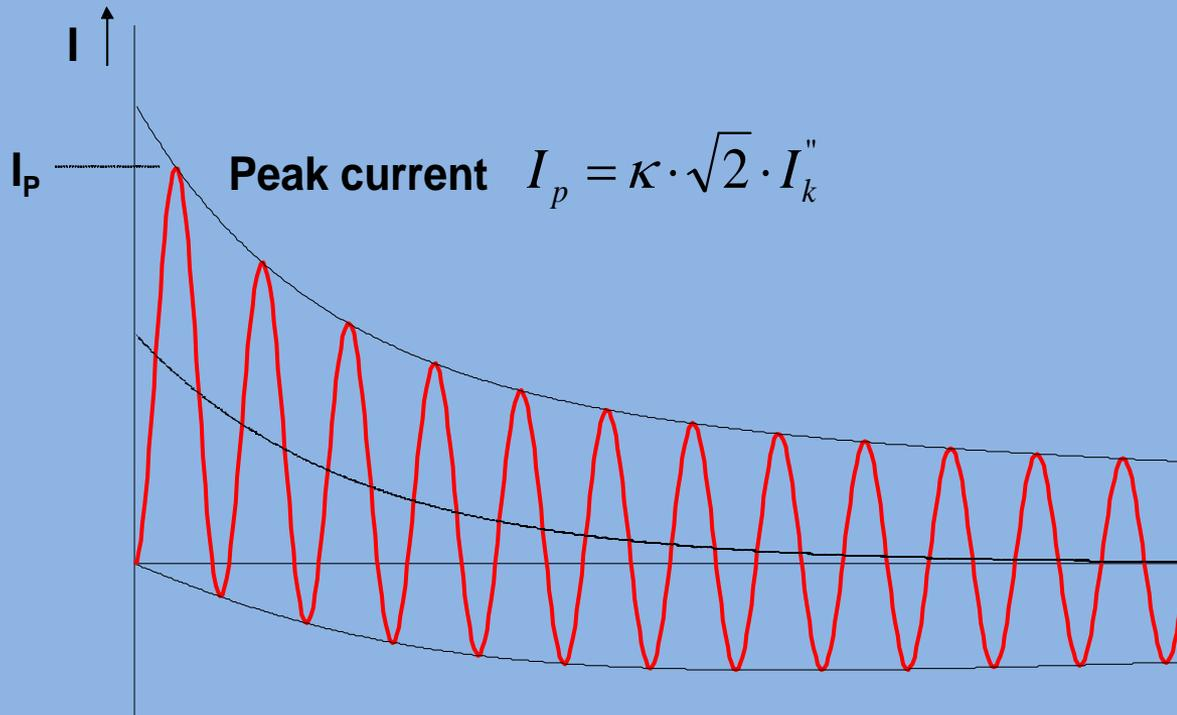
**IEEE:**  $I_{ma}$  or  $I_p = 2,6 \cdot I_k$  at 60 Hz
