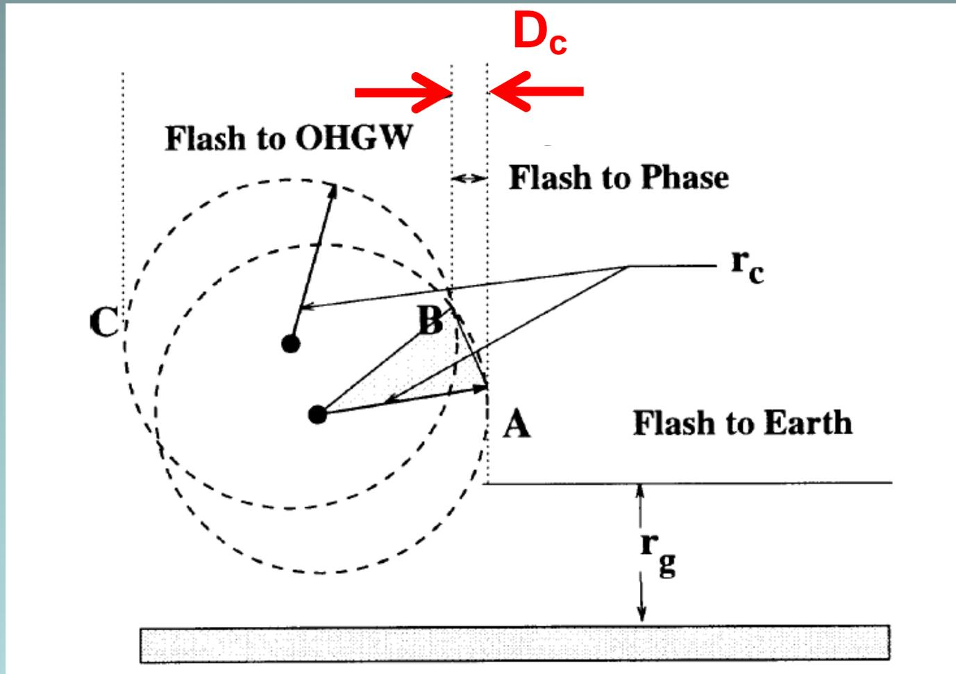
**$D_c$  - Exposure Distance for a shielding failure**
