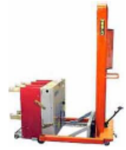
2. Roll Circuit Breaker on Truck Lift
