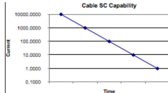
$$\left[ \frac{I_{SC}}{A} \right]^2 t = 0.0297 \log_{10} \left[ \frac{T_2 + 234}{T_1 + 234} \right]$$
