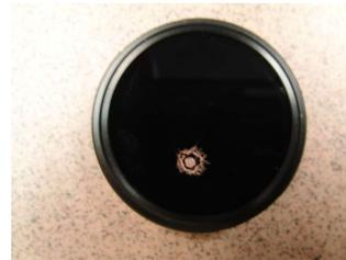
Lens was damaged by the melted copper
