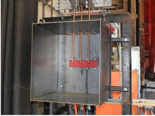
**Vertical Electrodes in the Enclosure (VCB)**
