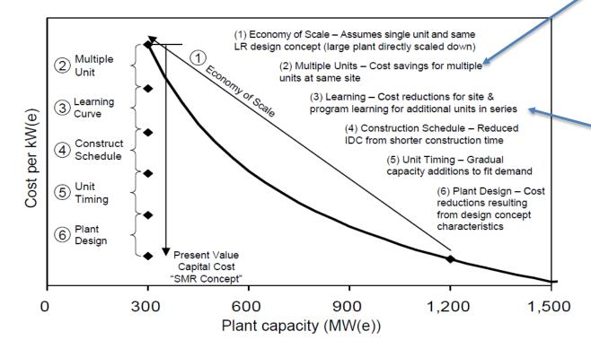
(2) SMRs are often designed to be built in sets. Sometimes with multiple reactors sharing key systems such as the turbine system or control room.
