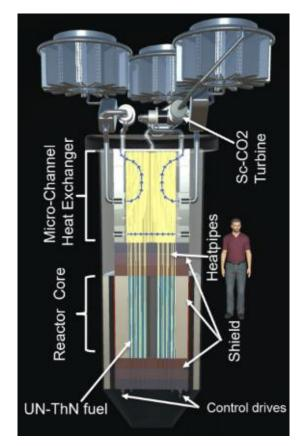
Smallest SMRs with power ratings <10 MWe\* are called Very Small Modular Reactors (VSMRs) or Microreactors.
