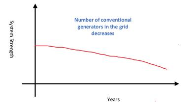
Weak grid condition can pose challenges for connecting new resources and particularly for connecting IBRs.
