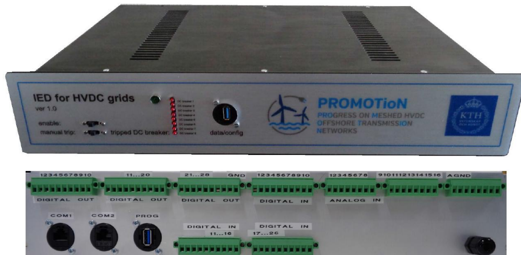
Fig. 73. Intelligent electronic device developed in EU Horizon2020 Promotion project. https://www.promotion-offshore.net/
