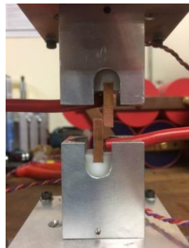
Figure 14. 400A DC current interruption with LC DC Circuit Breaker.
